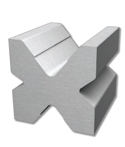
US 209/4V dimensioni-dimensions 60x60 mm cava V - slot V 16-22/88° 35-50/85° C45 rettificato-grinding temprato ind.-induction hardened HRC 52/58 lunghezze-lengths 835 mm - 415 mm - fraz
